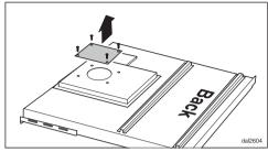
■ Remove the small cover on the rear of the ventilation system.
